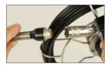
To connect, align the arrow on the bayonet jack with the arrow on the bayonet plug. Then mount the camera head onto the end of the GRP rod and secure it using the union nut.
