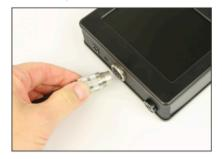
Connect the 8-pin plug of the cable to the socket on the monitor. Tighten the connection by hand.
