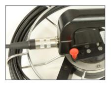
Also connect the socket and plug at the handle by inserting them straight and tightening the connection by hand.
