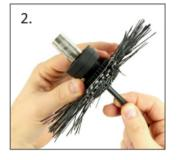
Screw the upper part on about 2 turns and feed the camera cable through.
