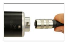
Connect the jack of the camera to the 8-pin connector on the camera head. Please make sure that the groove guide of the plug matches with the socket. Screw the plug with the threaded screw tight.
