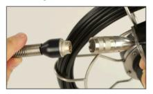
Connect the socket of the camera rod (or cable) to the plug on the camera head. Hand-tighten the screw connection. Only switch on the monitor once everything is connected. The system must be started as a complete unit; otherwise, no video signal will be received.
