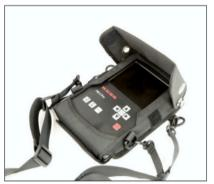
After sliding the monitor into the protective case, close the bottom using the hook-and-loop fastener.
