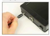
The monitor can be operated either via the battery or the power adapter. When the power adapter is connected, an "L" appears in front of the percentage display. The device can be used while the battery charges simultaneously. The status LED lights up red during charging. Once the battery is fully charged, it turns green.
