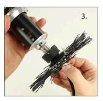
First, screw the plug of the camera cable onto the camera head. Then insert the upper part of the cable gland into the groove. Only now tighten the lower part, making sure that the locking pins engage properly.
