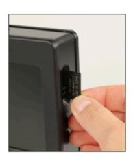
Insert the SD-card with the writing on top until you hear a "click". Now the SD-card is locked and ready to be used. To remove, please push the SD-card until you hear a "click" again. The card will pop out automatically. Now it can be connected to a reading device (not supplied).
