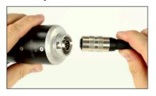
Connect the socket of the camera cable to the plug on the camera head. Hand-tighten the screw connection. Only switch on the monitor once everything is connected. The system must be started as a complete unit; otherwise, no video signal will be received. The Rotary-Ball-Camera is controlled using the arrow keys on the FM5 Pro monitor. The SK7 uses joystick control.
