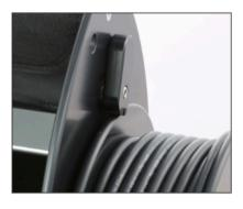
The fixing brake clamps the cable to prevent an unwinding during an inspection or transporting. Always clamp the cable with the fixing brake, before letting go of the cable during an inspection.
