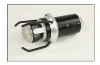
Slide the protection basket, with the guard brackets facing forward, over the housing of the pan-tilt camera until it reaches the stop ring. Then carefully secure it with the screw.
