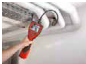
Inspection of hollow spaces
