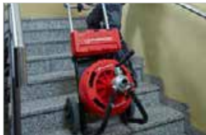
Easy transport due to stair capable chassis
