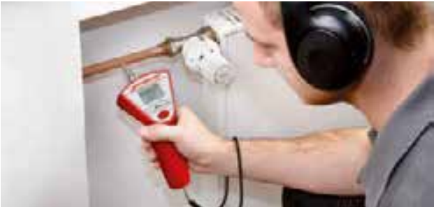
Acoustic leak detection of heating installations
