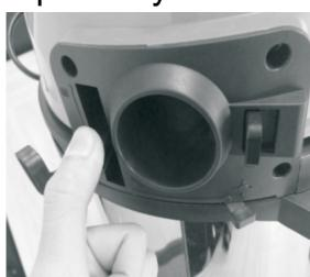
The connection method for blowing function.
