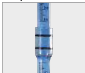
Transparent tube element with double o-ring seal
