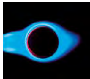
High flame temperature based on cyclone swirl
