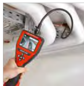
Inspection of hollow spaces
