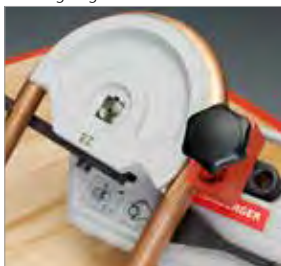
Forged aluminium segments with bending angle scale
